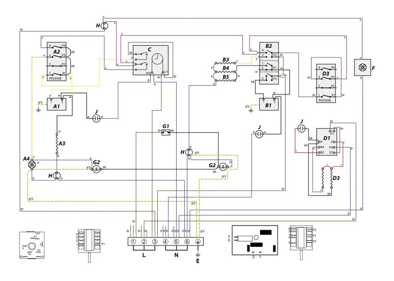
*Key*The connections shown in the circuit diagram are for single-phase. The ratings are for 230V 50Hz.
